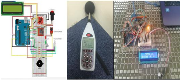
Figure 4. Outlining assembly of an Arduino, SLM 3M Pro type II, Microcontroller
